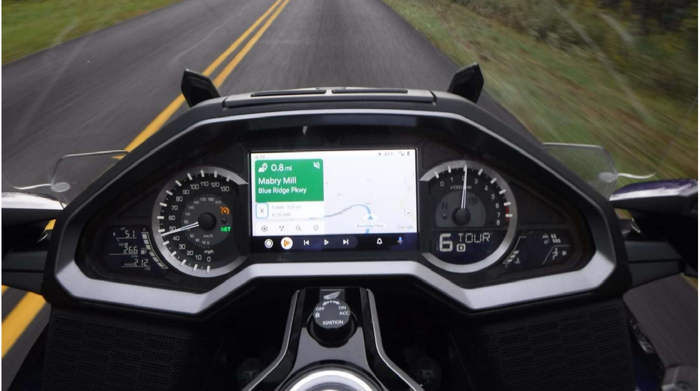
Figure 1 This is the actual instrument cluster with Android Auto on the screen.
